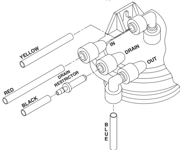
2. Locate the  $\frac{1}{4}$ " Red Feed Water Tubing. Remove the red plug from the fitting labeled "In" on the manifold and insert the tubing. Reference the special supplement sheet in the carton for proper connection of all tubing and removal of plugs. Run the tubing along its course to the Feed Water Saddle Valve, trim to length. (Refer to Fig. 1.)
