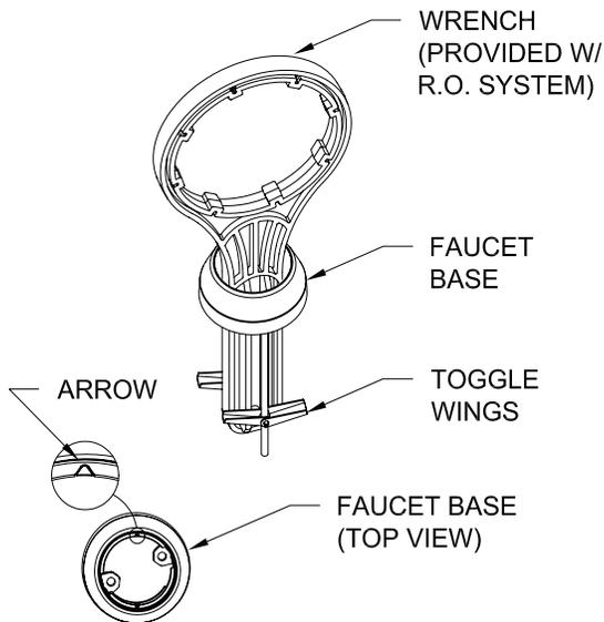
4. Place the Base Assembly through the mounting hole on the sink or counter top.
